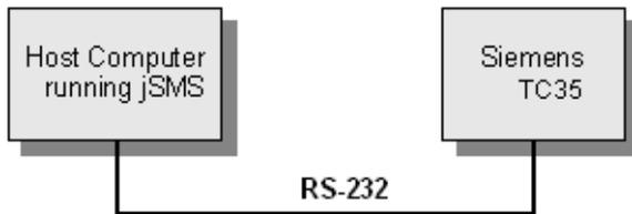
The GSM Device (e.g. your Mobile Phone) is connected **directly to a serial port** on the host computer. The jSMS API will communicate with the device using a **javax.comm** compliant library.
